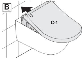
Press C-1 into A-6 until C-1 engages with a click. (After C-1 is mounted, make sure that it cannot be removed even if it is pulled.)
