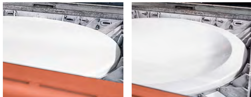
The acrylic sheets are heated and vacuum-drawn into the mould. Once cooled, the moulded object is then precisely ground and polished.
