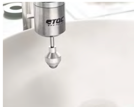
Its particular robustness has been demonstrated by the falling ball test.
