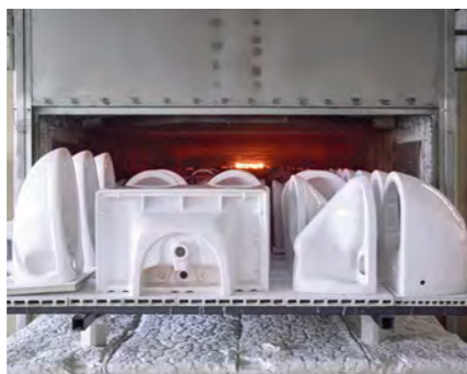
The glazed blanks are placed for approx. 16 hours in furnaces heated to as much as 1,200 °C to produce the finished product.
