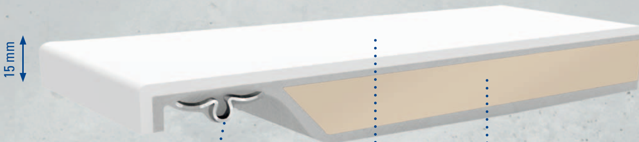
CROSS SECTION OF SHOWER TRAY, RIM HEIGHT 15 MM
