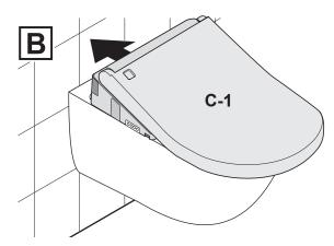
Press C-1 into A-6 until C-1 engages with a click. (After C-1 is mounted, make sure that it cannot be removed even if it is pulled.)
